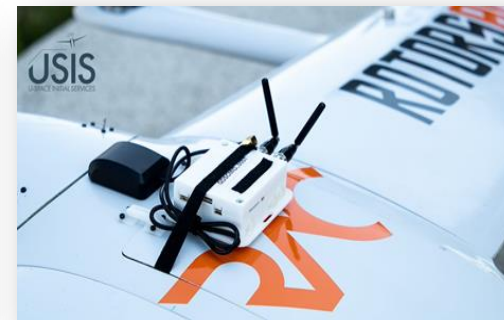
Drone Secure Communications Module Secure connectivity – encrypted signature; GPS Rx; IoT Module & embedded e-SIM
